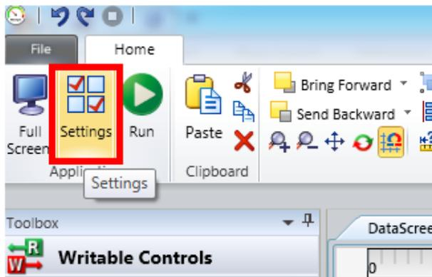
13. In the  $\mu$ C/Probe setting window, select the Cypress PSoC Prog and select 'KitProg/<Kit Prog number>' from the drop down box for Port and click **OK** to start communication between the CY8CKIT-042 and the  $\mu$ C/Probe tool.
