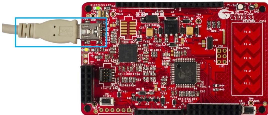
2. The onboard PSoC 5LP uses serial wire debug (SWD) to program the PSoC 4 device. See [Figure 3-4](#) for this implementation.
