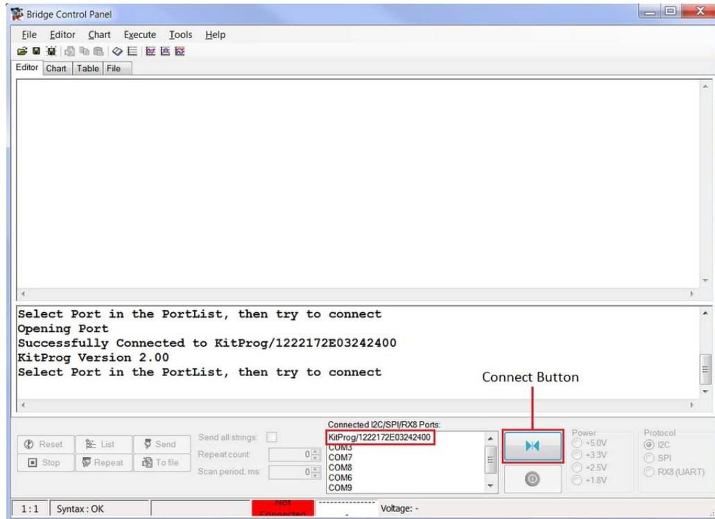
To use the USB\_I2C functionality, select the **KitProg/<serial\_number>** in the BCP. On successful connection, the **Connected** and **Powered** tabs turn green.
