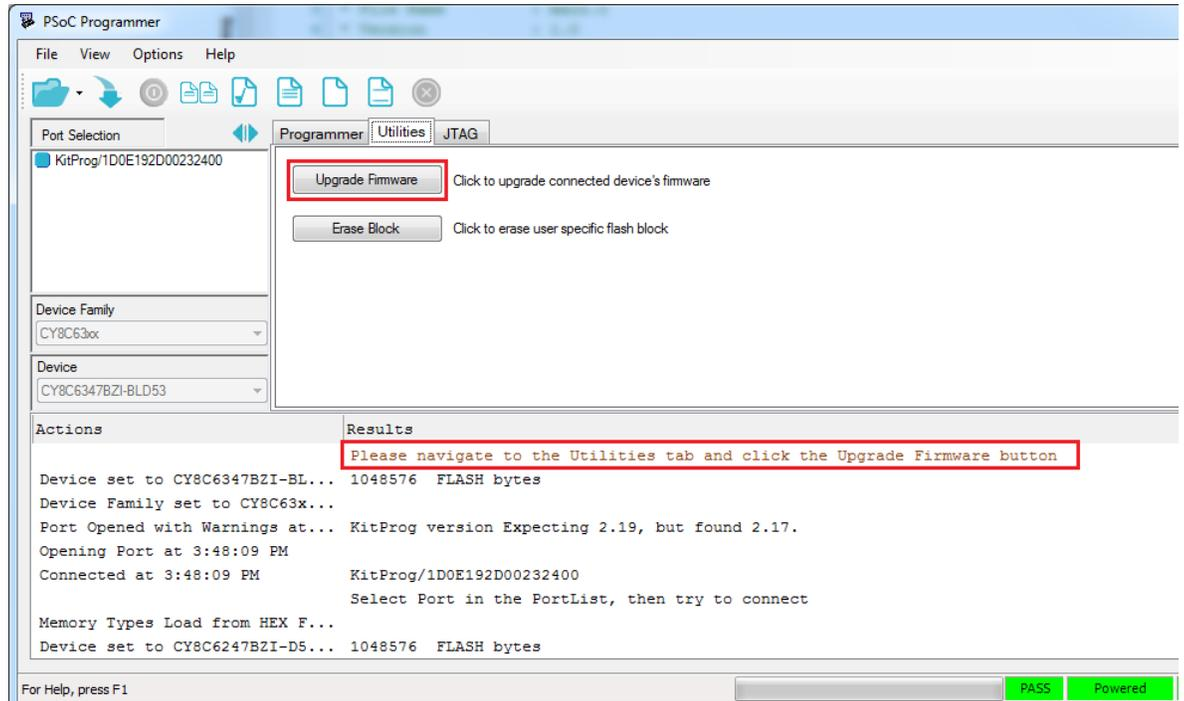
Click the **Utilities** tab and click the **Upgrade Firmware** button. On successful upgrade, the **Action and Results** window displays the firmware update message with the KitProg version.
