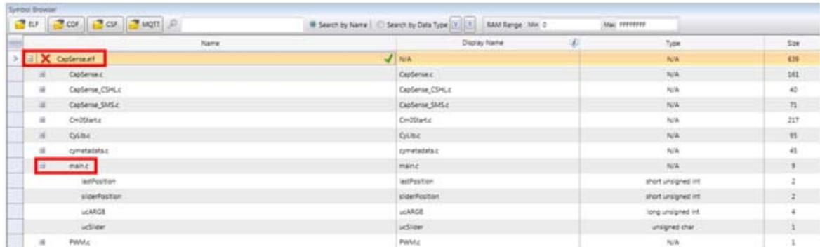
11. Drag and drop the global variable `ucSlider` on to the custom slider control to see the slider output. Similarly, drag and drop the global variable `ucARGB` on to the RGB Palette to see the RGB output.
