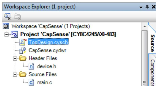
2. To open the tuner, right-click on the CapSense\_CSD component in PSoC Creator and click **Launch Tuner**.
