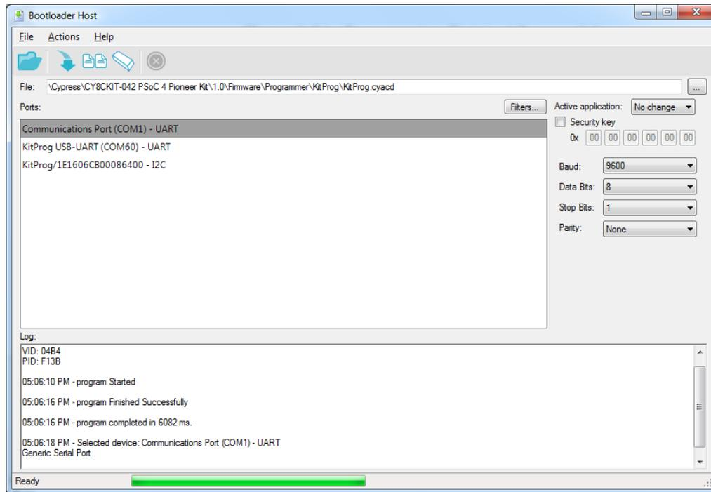
7. The factory program is now successfully restored on the PSoC 5LP. It can be used as the programmer/debugger for the PSoC 4 device.
