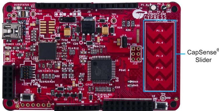
Figure 4-14. CapSense Slider Connection
