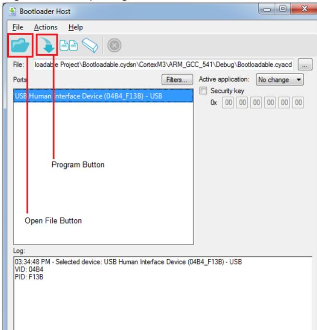
11. Press the **Program** button in the Bootloader Host tool to program the device.
