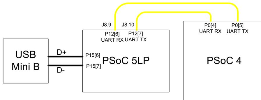
**Note:** UART RX and UART TX can be routed to any digital pin on PSoC 4 based on the configuration of the UART component. An SCB implementation of UART will route the RX and TX pins to either one of the following subsets: (P0[4], P0[5]) or (P3[0],P3[1]) or (P4[0],P4[1]).
