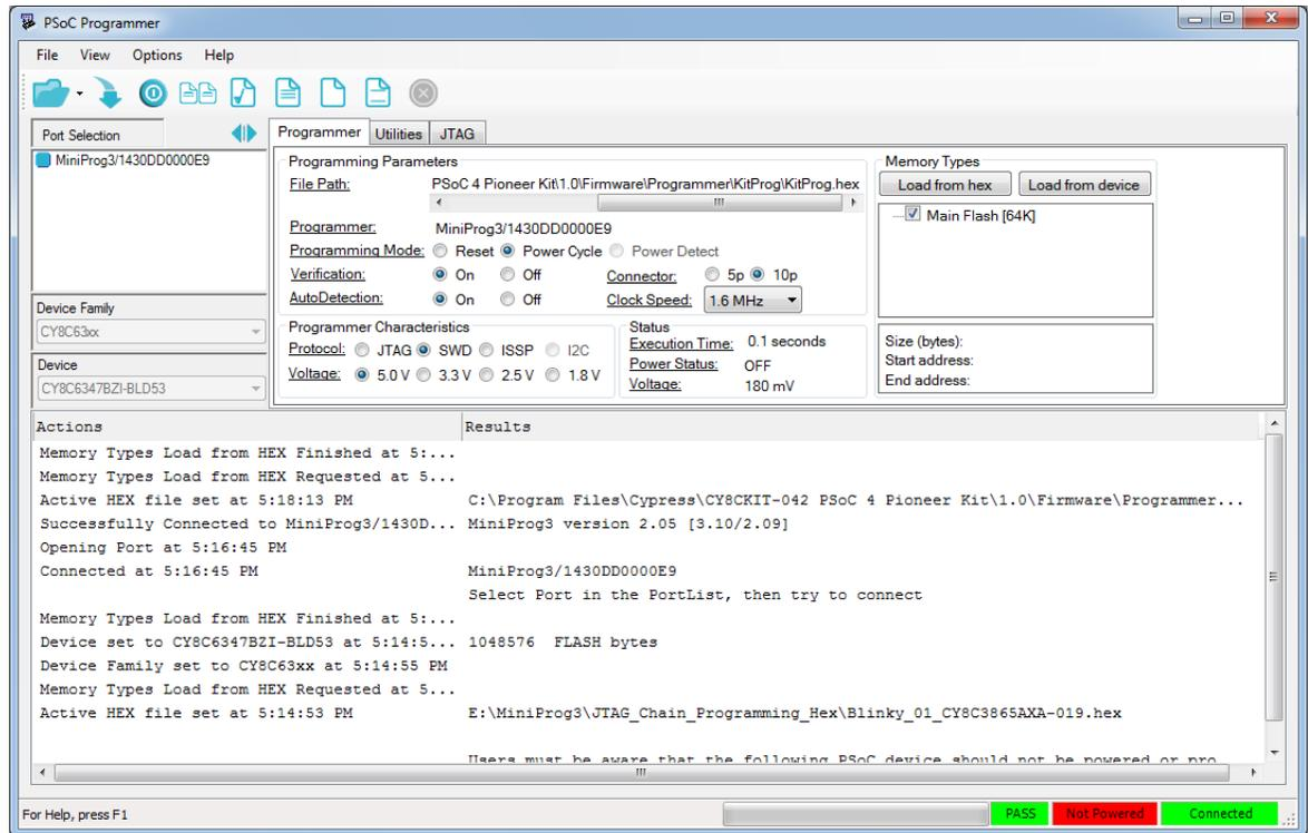
5. When ready, press the **Program** button (or **File > Program**) to program the PSoC 5LP device.
