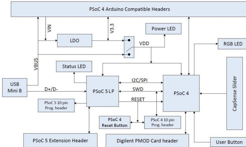
The PSoC 4 is a new generation of programmable system-on-chip devices from Cypress for embedded applications. It combines programmable analog, programmable digital logic, programmable I/O, and a high-performance Arm Cortex-M0 subsystem. With the PSoC 4, you can create the combination of peripherals required to meet the application specifications.
