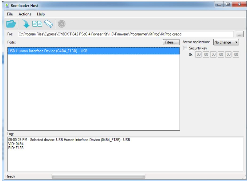
5. Click the **Program** button (or menu item **Actions > Program**) to restore the factory-program by bootloading it onto the PSoC 5LP.
