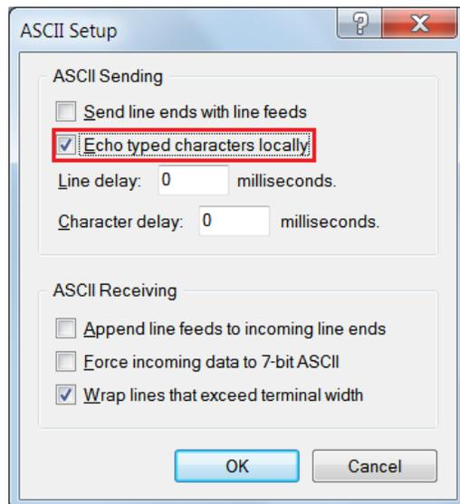
Figure 6-18. Enabling Echo of Typed Characters in PuTTY
