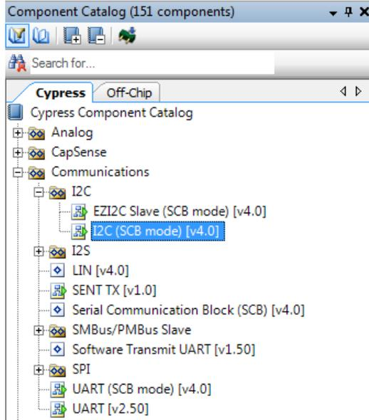
3. To configure the I2C component, double-click or right-click on the I2C component and select **Configure**.
