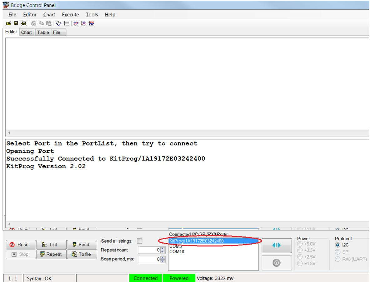
9. Open **Protocol Configuration** from the **Tools** menu and select the appropriate **I2C Speed**. Make sure the I2C speed is the same as the one configured in the I2C component. Click **OK** to close the window.
