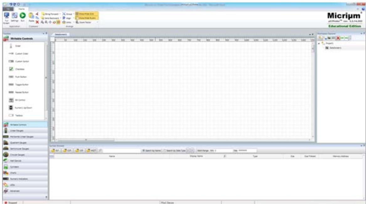
4. Drag and drop a Custom Slider control from Writable Controls in Toolbox on to the Datascreen1.
