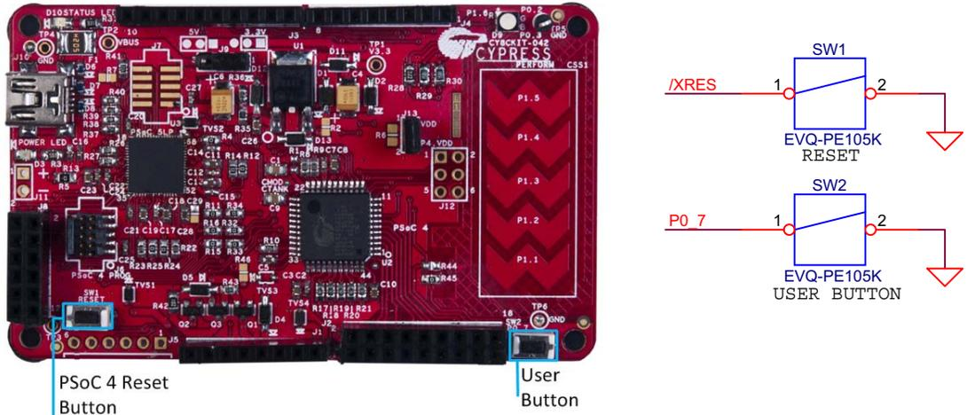
**Note:** The PSoC 4 Reset pin (XRES) has an internal pull-up resistor. However, an external pull-up resistor R10 is connected to the PSoC 4 Reset pin on the kit, which is optional and required only in a noisy system.
