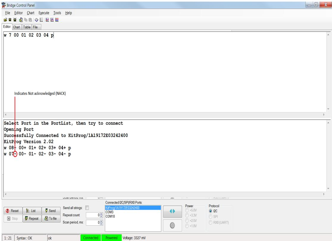
11. From the BCP, read five bytes of data from the I2C slave device with slave address 0x08. The log shows whether the transaction was successful.
