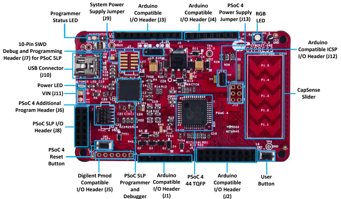
Figure 4-2. PSoC 4 Pioneer Kit Pin Mapping
