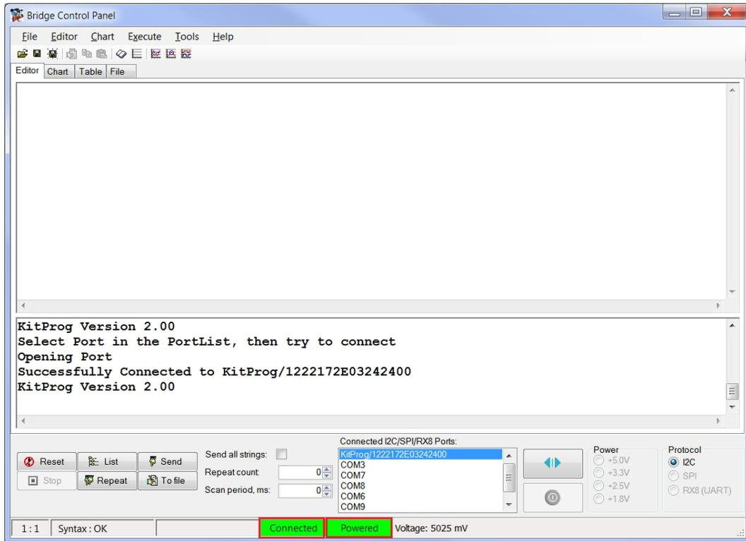
USB-I2C is implemented using the USB and I2C components of PSoC 5LP. The SCL (P12\_0) and SDA (P12\_1) lines from the PSoC 5LP are connected to SCL (P3\_0) and SDA (P3\_1) lines of the PSoC 4 I2C. The USB-I2C bridge currently supports I2C speed of 50 kHz, 100 kHz, 400 kHz, and 1 MHz.
