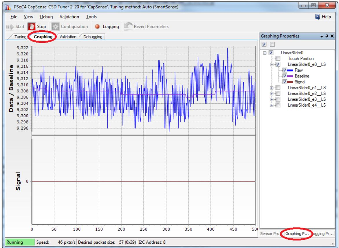
5. Touch a sensor or slider element and see the increase in raw counts.
