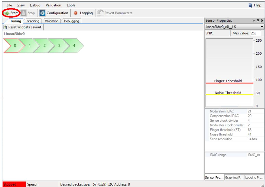
2. Select a sensor in the Tuning tab. A red outline is seen on the selected sensor. Different CapSense parameters are shown in Sensor Properties tab on the bottom-right. You cannot edit the settings because auto-tuning is used in this project; auto-tuning automatically sets all the parameters. Touch the selected sensor and observe the response in the tuner window.
