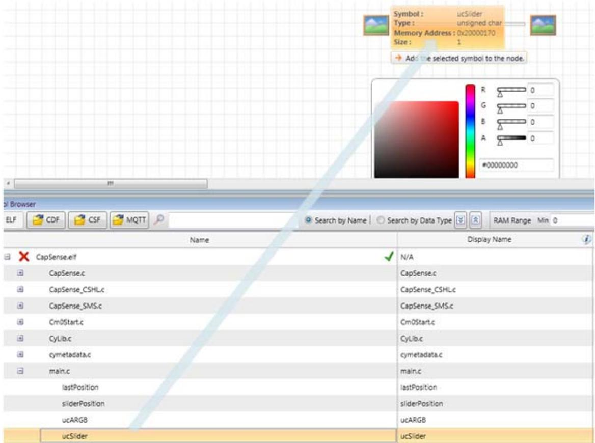
Figure 6-70. Assigning RGB output to RGB Palette control
