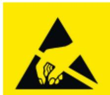
The CY8CKIT-042 contains electrostatic discharge (ESD) sensitive devices. Electrostatic charges readily accumulate on the human body and any equipment, and can discharge without detection. Permanent damage may occur on devices subjected to high-energy discharges. Proper ESD precautions are recommended to avoid performance degradation or loss of functionality. Store unused CY8CKIT-042 boards in the protective shipping package.
