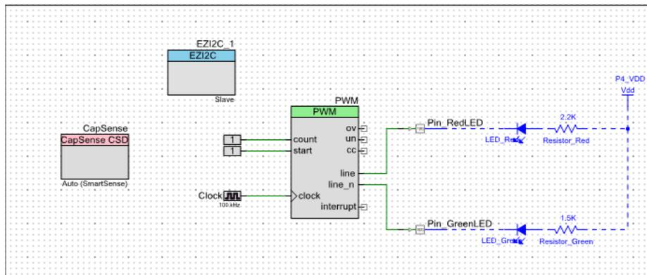
**Note:** The EzI2C component is not used when tuning is disabled.
